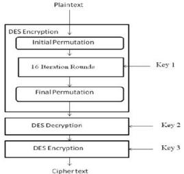
Fig 8 Internal operation of Triple Data Encryption Standard. The encryption algorithm is: Cipher text =  $E_{K3}(D_{K2}(E_{K1}(plaintext)))$  i.e., DES encrypts with K<sub>1</sub>, DES *decrypt* with K<sub>2</sub>, then DES encrypt with K<sub>3</sub>.Decryption is the reverse: Plaintext =  $D_{K1}(E_{K2}(D_{K3}(\text{cipher text})))$  i.e., decrypt with K<sub>3</sub>, *encrypt* with K<sub>2</sub>, and then decrypt with K<sub>1</sub>.
