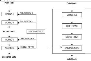
Fig 7. Internal operations of Advanced Encryption Standard. 3. *Triple Data Encryption Standard*
